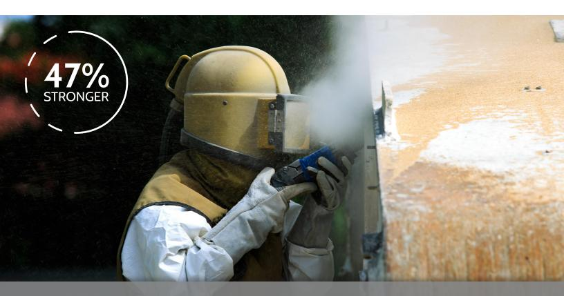
Iron Pillar Energy used Copper Slag to meet the challenge of maximizing its production rate at the lowest price point head-on. The switch to Copper Slag resulted in a production rate improvement of 47% for a significantly more powerful, more cost-effective blast.
